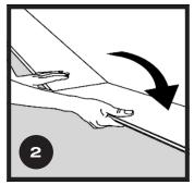
Second plank, first row. Drop the plank of short side first, and then gently tap down the end with a rubber mallet so it firmly locks into the previous plank until both are at the same height. Make sure both planks are perfectly aligned. Continue installing the first row until you reach the wall on the right.
