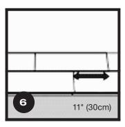
Make sure that end joints of all planks should be staggered 30cm at least or more.
