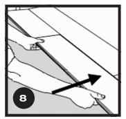
Drop the long side of the plank into the previous row and place it tight to the previous plank with an angle of 30 degrees, and gently tap on the end with a rubber mallet so it firmly locks into the previous plank until both are at the same height. Make sure both planks are perfectly aligned.
