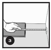
At the end of the first row, leave an expansion gap of 1/4" (6mm) to the wall and measure the length of the last plank to fit.
