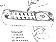
While holding the 'C' BUTTON, remove/add CODE (Red) and NON-CODE (Blue) Tumblers to create your desired code.
