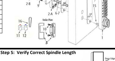
1. Hold the Inside Body (#2) and Rubber Inside Body (#2) Trim Plate (#3) to the door.
