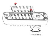
3. TURN & HOLD thumb-turn to right or left 90° to release tumblers. IMPORTANT: THUMB-TURN MUST be turned 90° and held when removing and inserting tumblers. Failure to do so will damage the lock and void the warranty.
