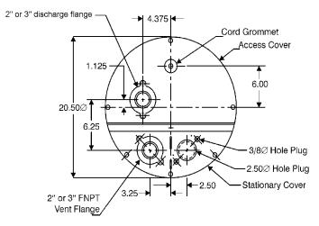
Cover Detail, One-Piece Cover 2" vent flange 4.50 5 stationary Cover 4.13 20.50% Cover 4.13 20.50% Cover Cover
