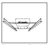
Ceiling mount - mounts to T-bar by adjustable bar hangers.
