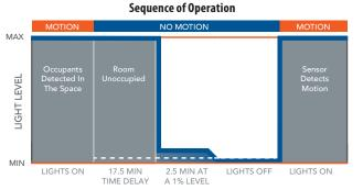
\*The presetting on the automatic dimming photocell is 5fc.
