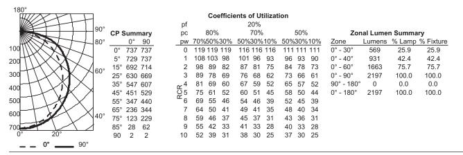
2VTL2 33L ADP L835, 3564 delivered lumens, test no. LTL24790P4, tested in accordance to IESNA LM-79
