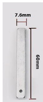
10.) Spindle for Door Thickness 35mm-55mm (1 3/8''-2 1/8'') (1)
