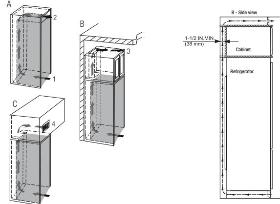
If the appliance is integrated in a fitted kitchen, the following ventilation requirements must be met: - The spacing fins on the back of the appliance are used to ensure sufficient ventilation. These must not lie in cavities or recesses in their final installation position. - Basically, the larger the ventilation gap, the more energy the appliance saves during operation. Do not restrict the air flow.
