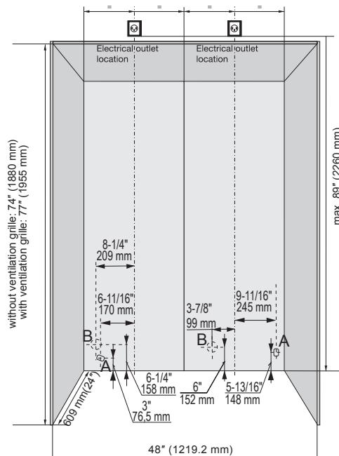
The appliances can be used freestanding or semi built-in. If semi built-in, consider the minimum cabinet opening dimensions specified on this image.
