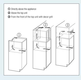
IMPORTANT When using decor grills, the sum of the individual openings must total a minimum of 31 square inches. A cut-out section of 31 square inches (200 cm<sup>2</sup>) for installing the ventilation grill is thus not sufficient.
