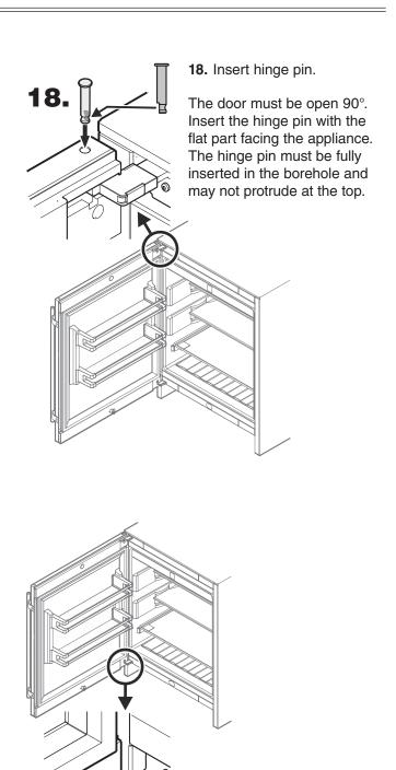
**19.** Insert the bottom hinge pin in the same way.
