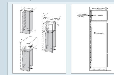
This type of cabinet must be carefully constructed using the correct dimensions and it must provide suitable ventilation to ensure proper appliance operation.
