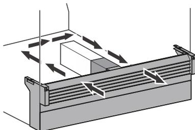
After installing the kitchen cabinet door, there must be a ventilation gap between the appliance ventilation grille and the kitchen cabinet door. The ventilation grille is movable to guarantee sufficient ventilation.
