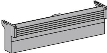
*The foam block supplied must be installed in order to ensure the required air flow through the appliance base.*
