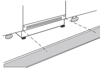
A cut-out in the toe kick panel is necessary when the toe kick covers the ventilation openings of the ventilation grille.
