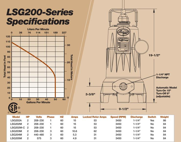
Single phase models are thermally protected. 3-phase models require a properly sized control panel. Maximum fluid temperature 140° F
