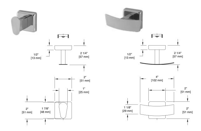
**MATERIALS:** Inner Wall Flange - 16 gauge type 304 stainless steel
