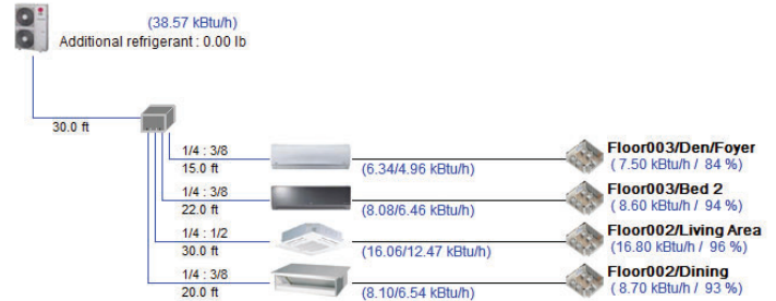
Figure 1: LATS Example (Tree Diagram; Illustrative Purposes Only. System will Vary Depending On Modell).
