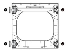
With the hinges and cover caps in the new locations, remount the inner door frame onto the outer door frame with the screws removed in step 3 above.
