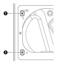
While supporting the door, remove the 2 screws **2** on the door hinge, two from each hinge. Set the door aside face down on a protected surface to prevent damage to the door or the work surface.
