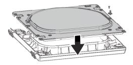
Reinstall the door with the screws removed in step 2. Install the two plastic hole caps removed in step 1 on the opposite side.
