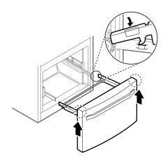
Lower the door into its final position and insert the screws in the rails on both sides.
