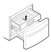
Remove the Durabase basket from the rails. Remove the screws from the rails at both ends.
