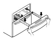
Pull the drawer open to full extension. Lower the basket onto the rails.
