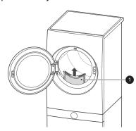
Always ensure the lint filter is properly installed before running the dryer. Running the dryer with a loose or missing lint filter will damage the dryer and articles in the dryer.
