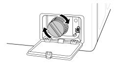
**8** Close the drain pump filter cover.
