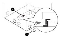
3 Preassemble a 4" (10.2 cm) elbow 5 to the next 4" (10.2 cm) duct section, and secure all joints with duct tape. Be sure that the male end of the elbow faces AWAY from the dryer. Insert the elbow/duct assembly through the side opening and press it onto the adapter duct. Secure it in place with duct tape. Be sure that the male end of the duct protrudes 1.5" (3.8 cm) to connect the remaining ductwork. Attach the cover plate 6 to the back of the dryer with the included screw.
