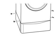
6 Extend all 4 feet 1 of the washing machine slightly until it is snugged up against the pedestal. Then tighten the four lock nuts 2.
