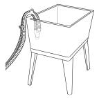
**3** Use the provided tie strap to secure the drain hose in place.
