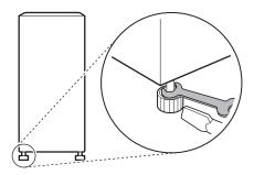
Open the door, and check to make sure that they close easily. If the door do not close easily, tilt the refrigerator slightly more to the rear by turning both leveling legs to the left. It may take several more turns, and be sure to turn both leveling legs the same amount.
