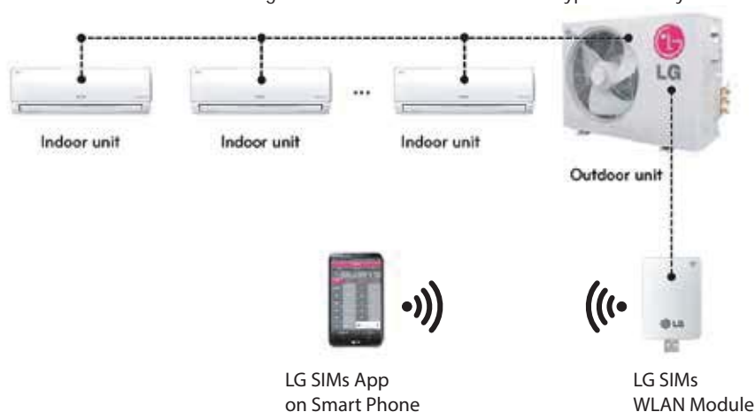
Figure 106: SIMS WLAN Module to Typical DFS System
