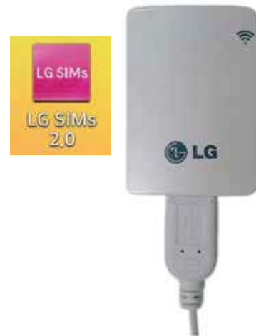
Figure 106: SIMS WLAN Module to Typical DFS System
