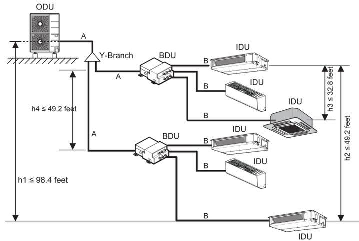
Example: LMU421HHV outdoor unit with six (6) indoor units and two (2) branch distribution units connected.
