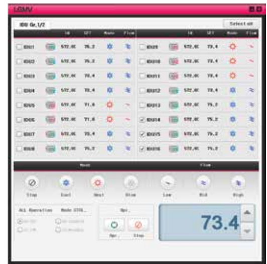
Figure 61: MV Control Indoor Units Screen.
