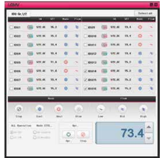
Figure 103: MV Control Indoor Units Screen
