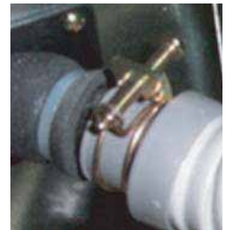
Clamp the Flexible Drain Hose Connection
