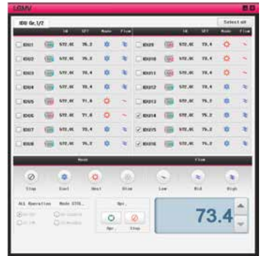
Figure 61: MV Control Indoor Units Screen.
