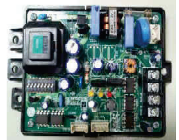
Figure 90: PI-485 Board (Appearance will differ depending on model).
