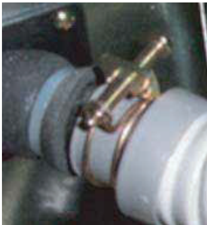
Clamp the Flexible Drain Hose Connection
