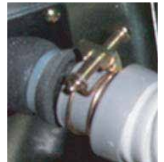
Clamp the Flexible Drain Hose Connection
