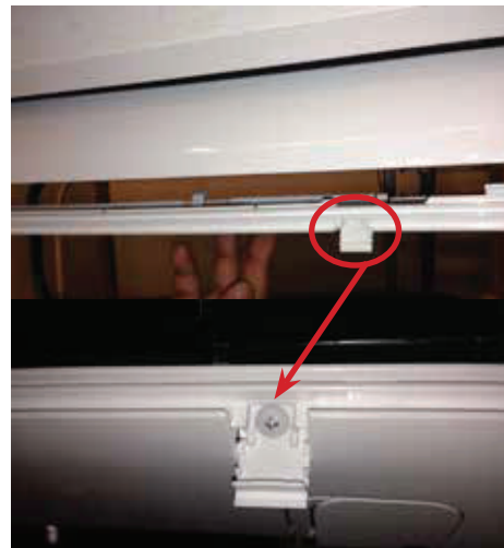
Figure 91: Reattaching the Screws on the Bottom Panel.
