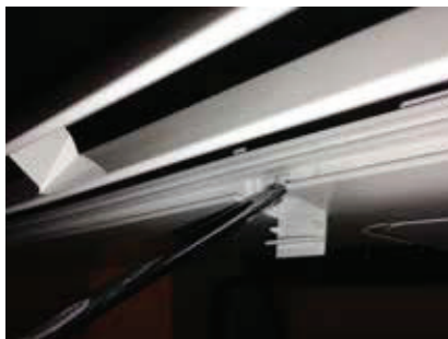
Figure 90: Reattaching the Screws on the Bottom Panel.
