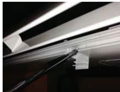
Figure 90: Reattaching the Screws on the Bottom Panel.
