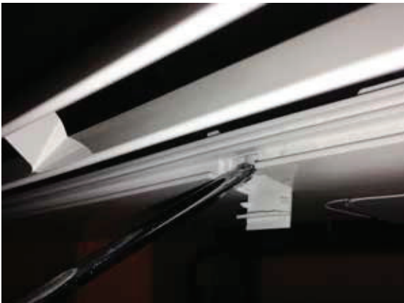
Figure 72: Remove Screws from Bottom Panel.
