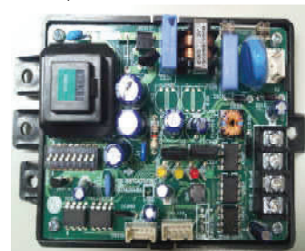
Figure 94: PI-485 Board (Appearance will differ depending on model).
