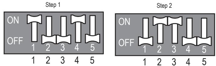
Figure 126: LMU360-420HHV Night Quiet Mode DIP Switch Settings.
