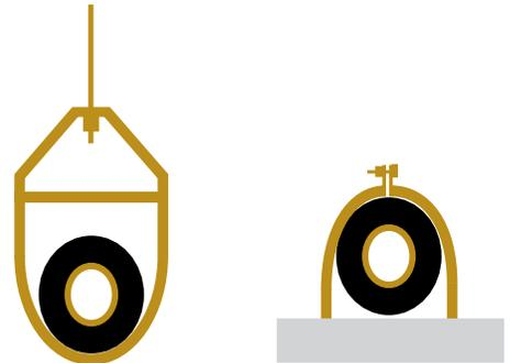
Figure 26: Typical Pipe Support Location—Change in Pipe Direction.
