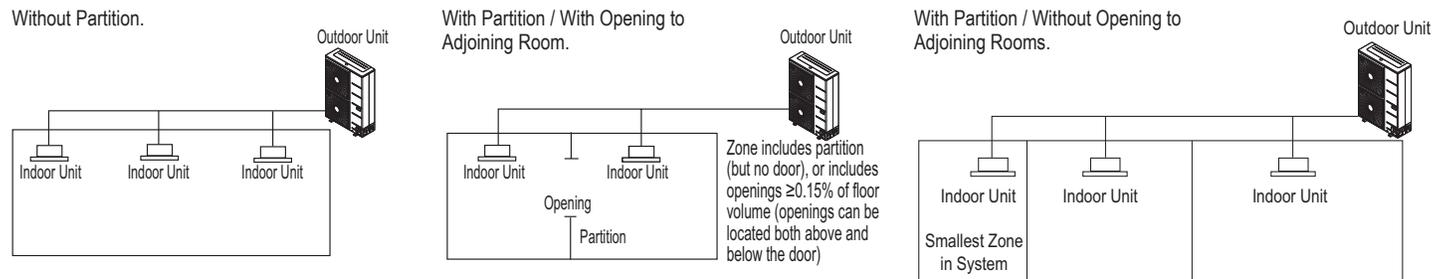
Figure 107: Example of Acceptable Ventilation Methods.
