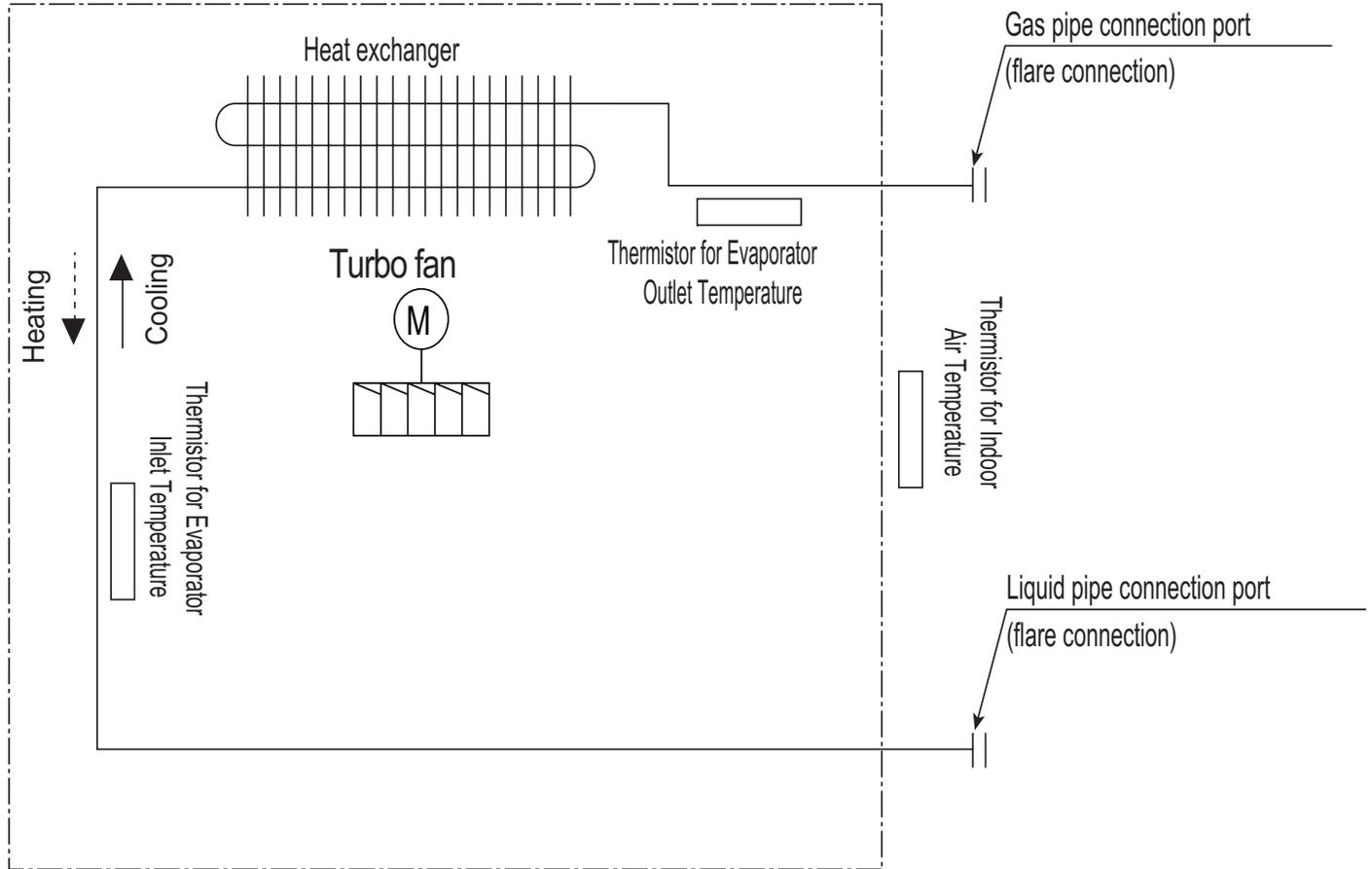
Table 6: Multi F Multi Zone Art Cool Mirror Wall-Mounted Indoor Unit Refrigerant Pipe Connection Port Diameters.
