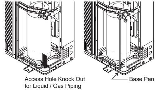
Figure 48: Filling Access Holes in the Outdoor Units.
