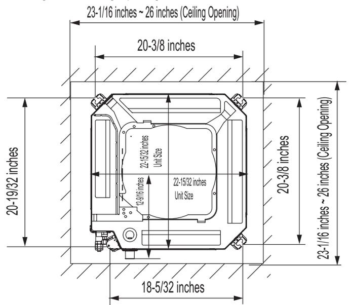
Figure 9: Installing the Hanging Bolt in the Ceiling.
