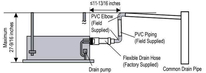
Figure 13: Drain Slope.
