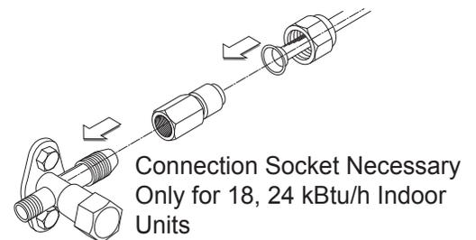
Figure 44: Connection Socket Diagram, External View.
