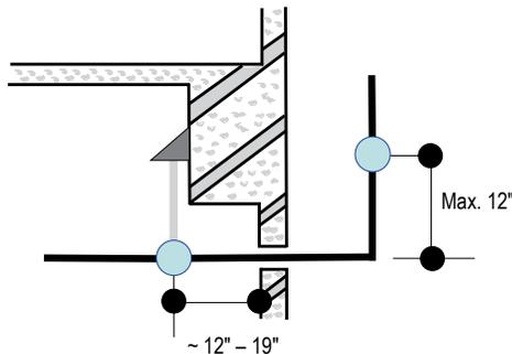
Figure 27: Pipe Support at Indoor Unit.
