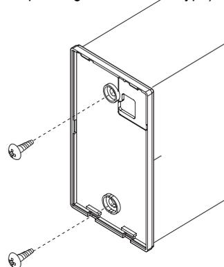
Figure 71: Installing / Removing the Controller.
