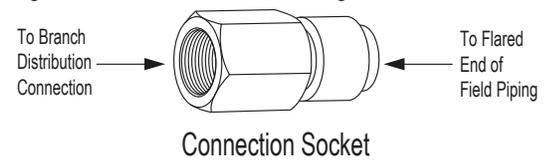
Figure 52: Close Up of Branch Distribution to Indoor Unit Piping Connections.
