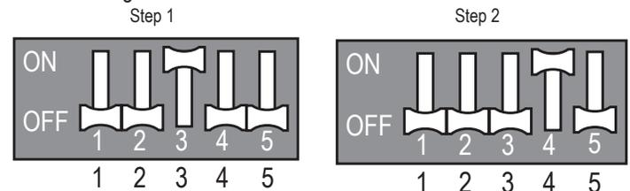
Figure 122: LMU360-420HHV Reducing Power Consumption DIP Switch Settings.
