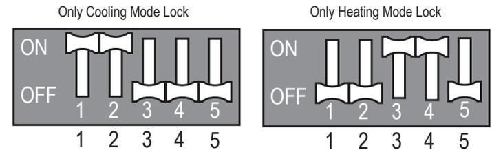
Figure 128: LMU360-420HHV Mode Lock DIP Switch Settings.
