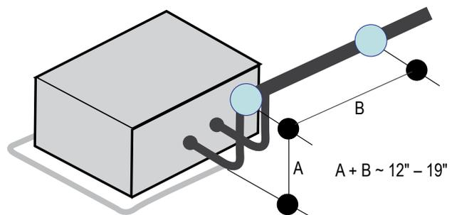
Figure 28: Pipe Support at Y-branch Fitting.
