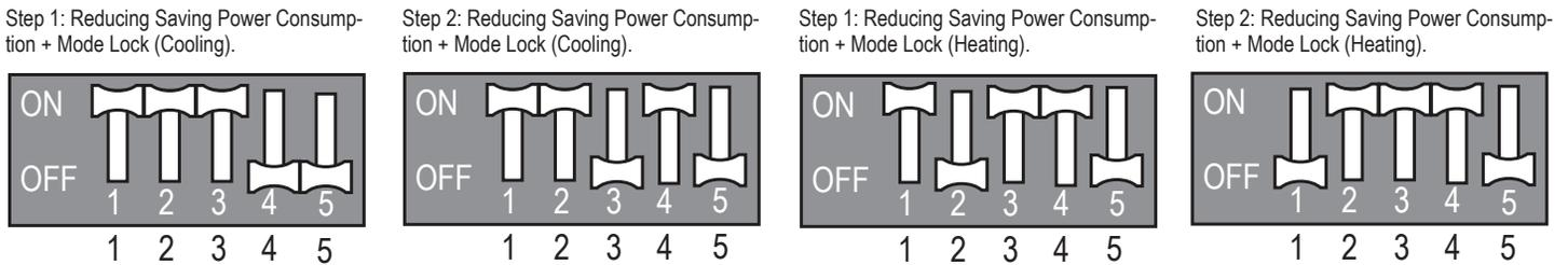
Figure 124: LMU360-420HHV Saving Power Consumption with Mode Lock DIP Switch Settings.
