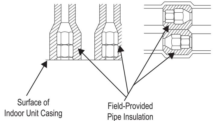
Figure 65: Insulating the Shut Off / Isolation Ball Valve (If Present).
