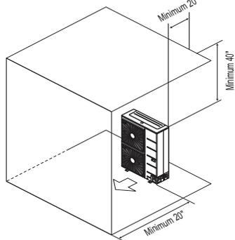
Where there are obstacles on both suction and discharge sides (discharge side obstacle is higher than the outdoor unit).
