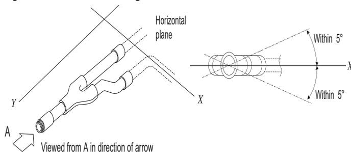
Figure 56: Y-Branch Port Identifier Diagram.
