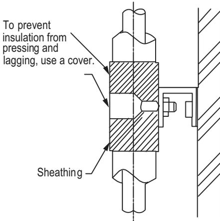
Figure 35: O-Ring Band Support with an Insulated Pipe.
