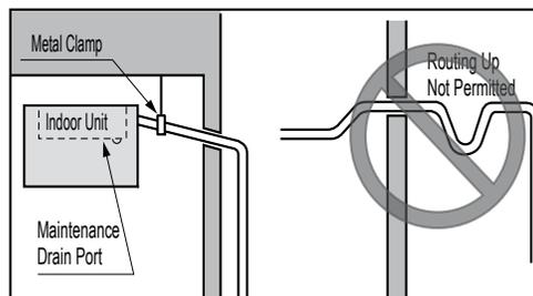
Figure 15: Flexible Drain Hose Connection.
