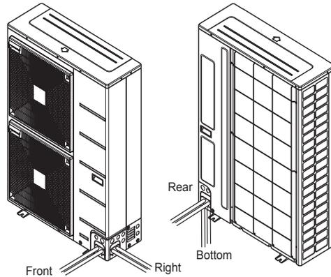
Figure 47: Removing the Base Pan Knock Out Hole.
