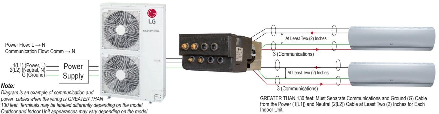
Figure 84: Multi F with LGRED LMU180HHV System Power Wiring and Communications Cable Connections.
