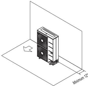
Obstacles on the suction side and on both left and right sides.
