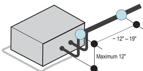
Figure 29: Pipe Support at Y-branch Fitting.
