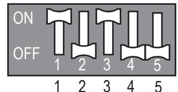
Figure 130: LMU360-420HHV Night Quiet Mode with Mode Lock DIP Switch Settings.
