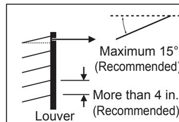
Figure 7: Using “S” Type Louvers.
