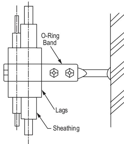
Figure 34: One-Point Down-Stop Support (>441 lbs.).
