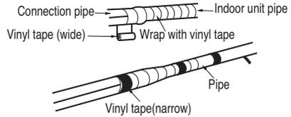
3. Bundle the piping and drain hose together by wrapping them with vinyl tape over the range within which they fit into the rear piping housing section.
