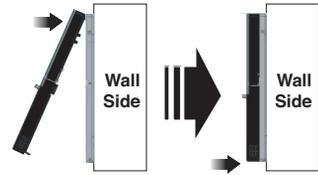
When separating remote controller from setup board, as the picture below, after inserting into the lower separating hole using screw driver and then, spinning clockwise, remote controller is separated.
