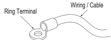
Figure 72: Adding a Ring Terminal to the Wiring.
