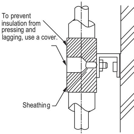
Figure 33: O-Ring Band Support with an Insulated Pipe.
