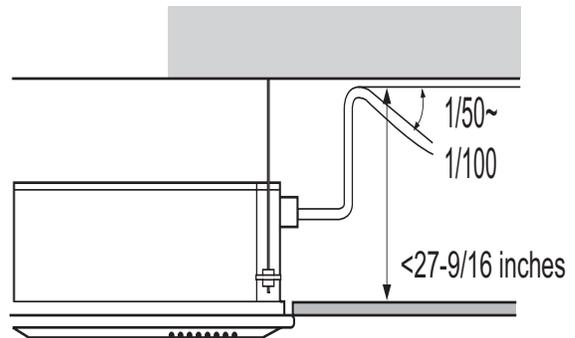
Figure 14: Correct (Another View) and Incorrect Drain Slopes.
