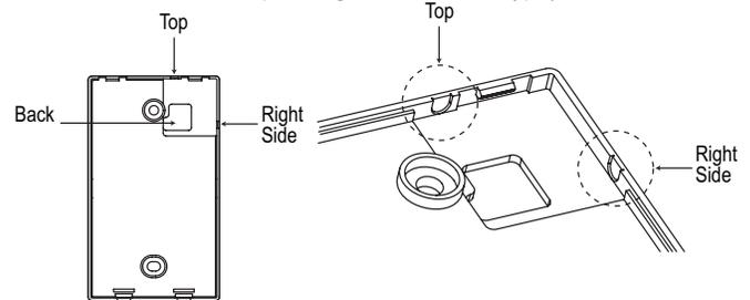
Figure 70: Attaching the Wall Plate (Plate Appearance will Differ Depending on Controller Type).
