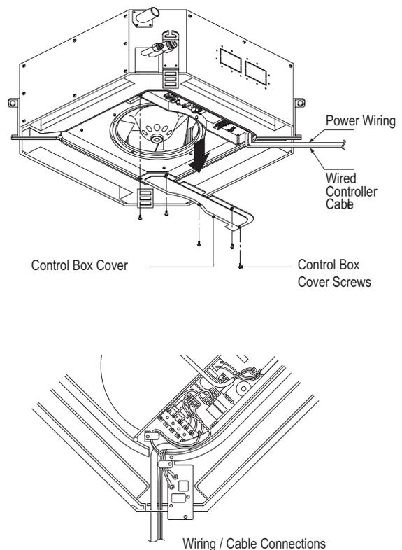
Figure 53: Simplified View of Indoor Unit to Outdoor Unit / Branch Distribution Unit Terminal Connections.
