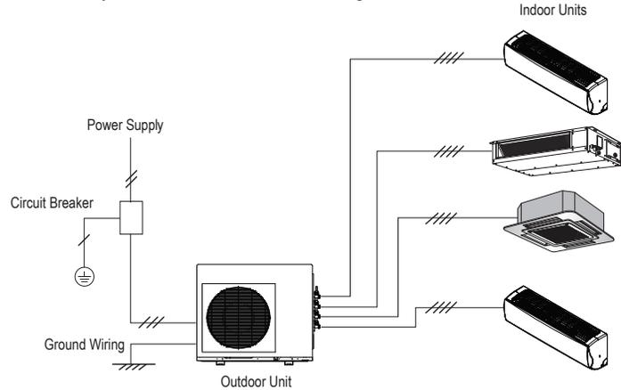
Figure 81: Typical Multi F MAX with LGRED System General Power / Communications System Schematic When Wiring is Less Than 130 Feet.
