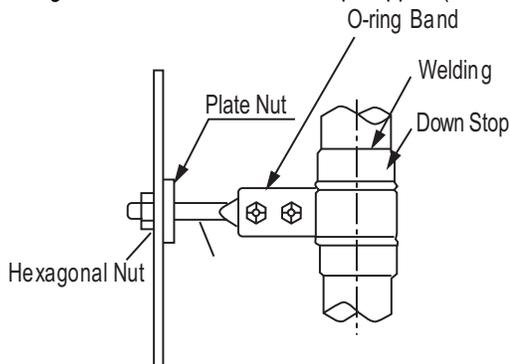
Figure 35: Two-Point Down-Stop Support.
