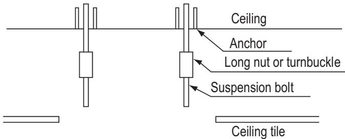
Figure 10: Installation Diagram.
