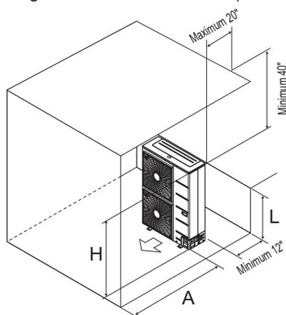
Where there are obstacles above, and on both suction and discharge sides (discharge side obstacle is lower than the outdoor unit).
