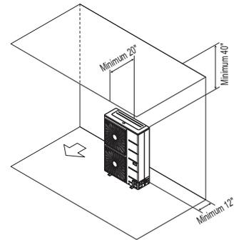
Obstacle on the suction side. Obstacles above, on the air intake side, and on both left and right sides
