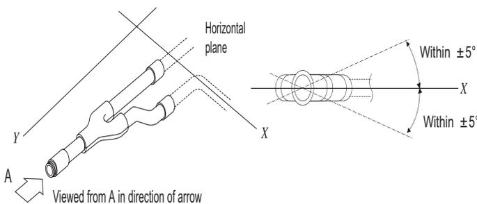
Figure 21: Y-branch Vertical Installation Alignment.
