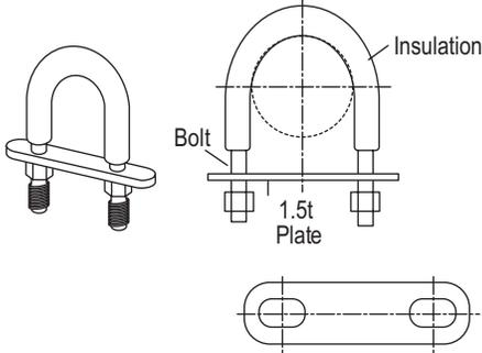
Figure 30: O-Ring Support with Insulation.
