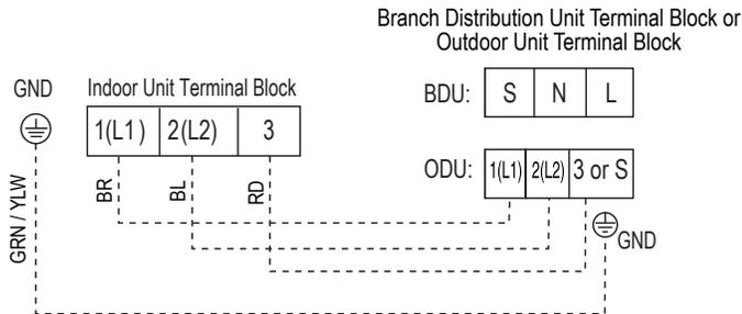
Figure 54: Typical Indoor Unit Terminal Block with Grounding Cable (Actual Appearance May Vary).
