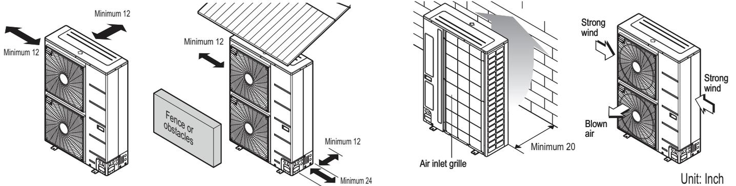
Ensure that the space at the back of the outdoor unit is a minimum of 12 inches, and include a minimum of 24 inches at the right side of the unit for service.
