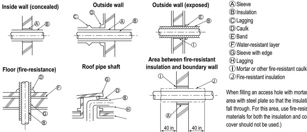
When filling an access hole with mortar, cover the area with steel plate so that the insulation will not fall through. For this area, use fire-resistant materials for both the insulation and cover. (Vinyl cover should not be used.)
