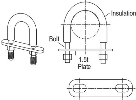
Figure 32: O-Ring Support with Insulation.
