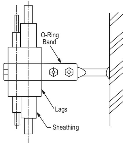
Figure 36: One-Point Down-Stop Support (>441 lbs.).
