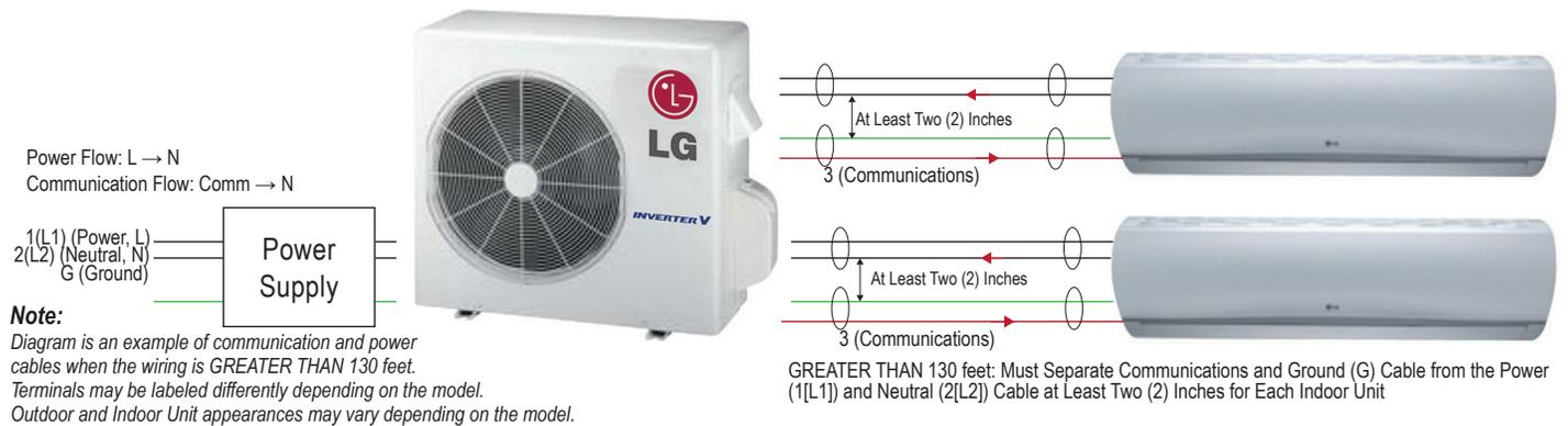
Figure 83: Schematic of a Multi F MAX with LGRED System When the Wiring is GREATER THAN 130 Feet.
