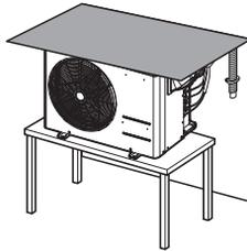
1. The height of H frame must be more than 2 times the snowfall and its width shall not exceed the width of the product. (If width of the frame is wider than that of the product, snow may accumulate)
