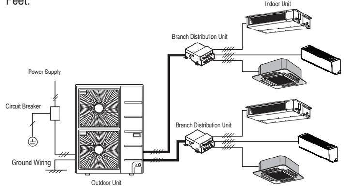
Figure 82: Schematic of a Multi F with LGRED System When the Wiring is GREATER THAN 130 Feet.
