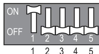
Figure 116: LMU360-420HHV Forced Cooling DIP Switch Setting.
