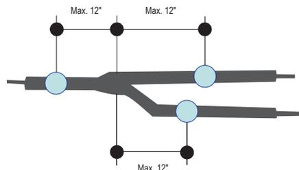
Figure 30: Pipe Support at Header Fitting.
