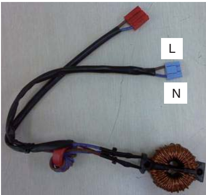
< Noise Filter wiring Check Point >
