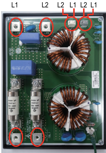
L1 L2 < Noise Filter wiring Check Point >
