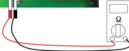
PFCM : Measuring resistance between No.19,20 pin
