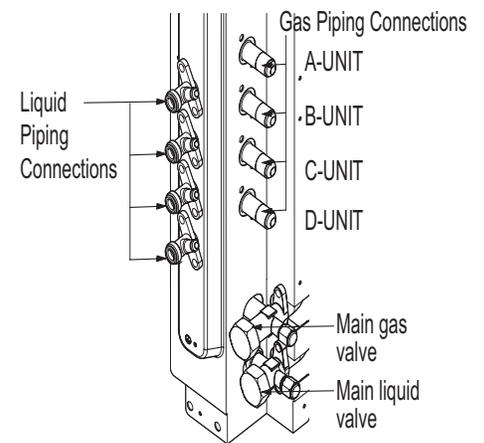
Connection sockets (included as a factory-supplied accessory with the indoor units) may need to be used when piping the indoor units to the outdoor unit.
