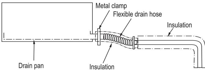
Figure 83: Diagram of an Indoor Unit with a Drain Pump.
