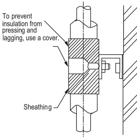
Figure 66: O-Ring Band Support with an Insulated Pipe.
