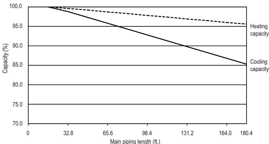
Table 160: Multi F MAX Branch Distribution Unit to Indoor Unit Refrigerant Line Length Derates.
