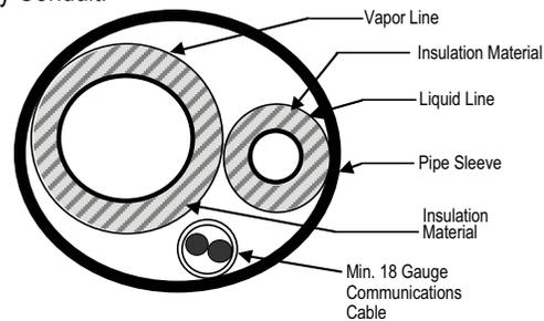
Figure 71: Underground Refrigerant Piping.
