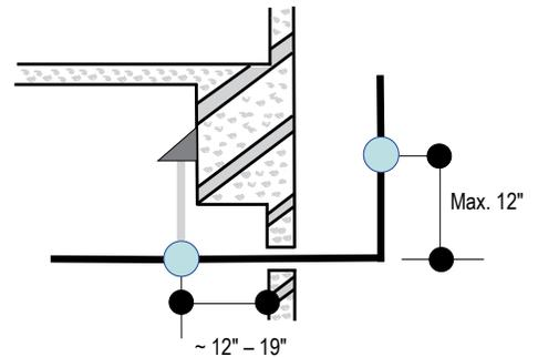
Wherever the pipe changes direction, place a hanger within twelve (12) inches on one side and within twelve to nineteen (12 to 19) inches of the bend on the other side as shown in Figure 59. Support piping at indoor units as shown in Figure 60. Support Y-Branch fittings as shown in Figure 61.
