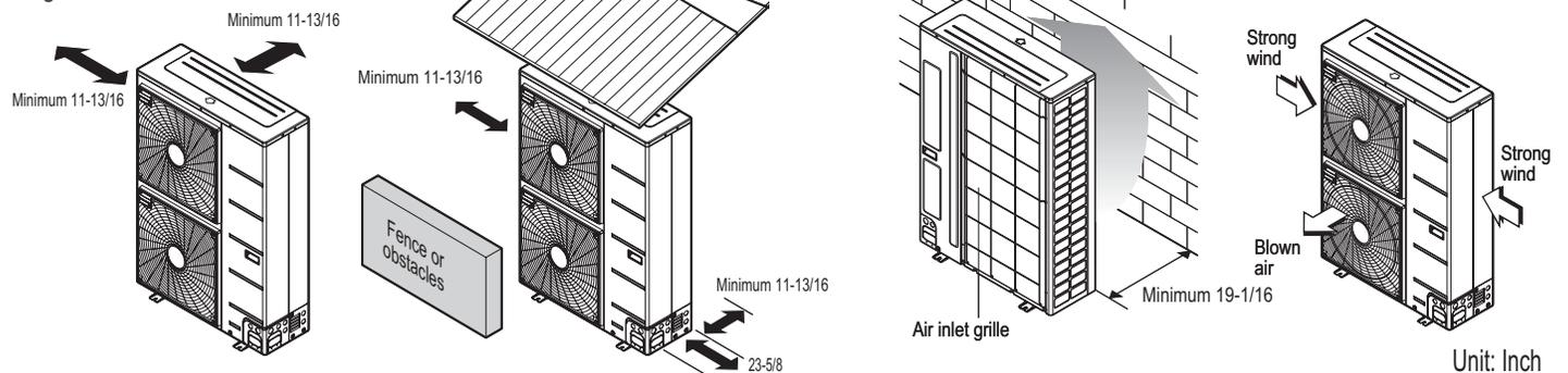
Ensure that the space at the back of the outdoor unit is a minimum of 11-13/16 inches, and include a minimum of 23-5/8 inches at the right side of the unit for service.
