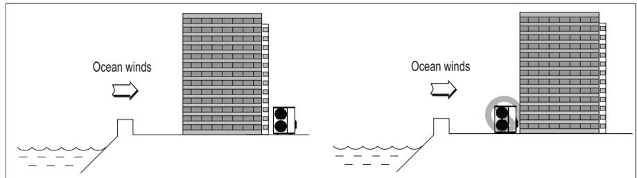
If the outdoor unit must be placed in a location where it would be subjected to direct ocean winds, install a concrete windbreaker strong enough to block any winds. Windbreaker height and width should be more than 150% of the outdoor unit, and be installed at least 27-1/2 inches away from the outdoor unit to allow for airflow.
