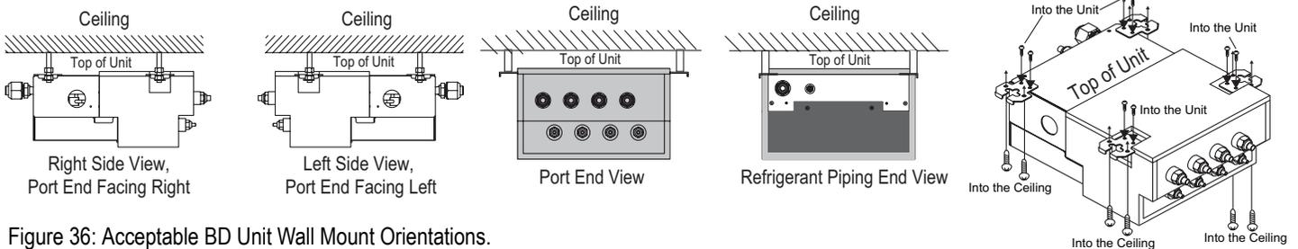
Figure 36: Acceptable BD Unit Wall Mount Orientations.
