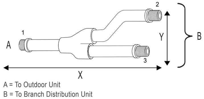
Multi F MAX Branch Distribution (BD) Units can be installed in a multitude of options to fit various building configurations and job or application requirements. Multi F MAX BD Units include electronic expansion valves that properly seat only if the BD Unit is installed in an acceptable orientation. Installations with improper BD Unit orientation risk incomplete valve seating and system performance degradation from potential refrigerant leakage through the electronic expansion valve.
