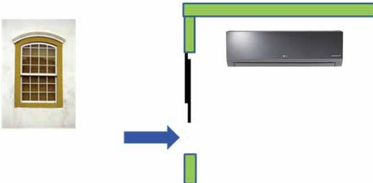
**Method 2: Unconditioned Outdoor Air (Non-Ducted, Fan Assisted Ventilation)**
