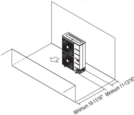
Where there are obstacles above, and on both suction and discharge sides (discharge side obstacle is lower than the outdoor unit).
