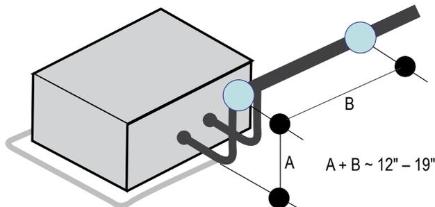
Figure 61: Pipe Support at Y-branch Fitting.
