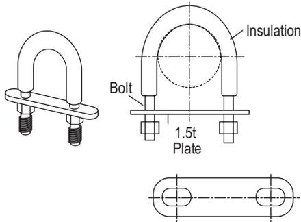
Figure 63: O-Ring Support with Insulation.
