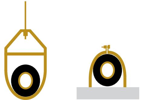
Field provided pipe supports should be designed to meet local codes. If allowed by code, use fiber straps or split-ring hangers suspended from the ceiling on all-thread rods (fiber straps or split ring hangers can be used as long as they do not compress the pipe insulation). Place a second layer of insulation over the pipe insulation jacket to prevent chafing and compression of the primary insulation within the confines of the support pipe clamp.
