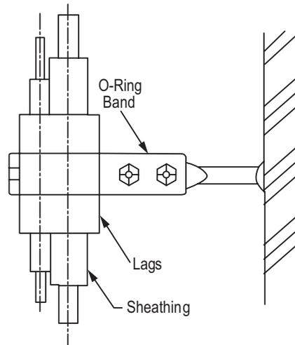
Figure 67: One-Point Down-Stop Support (>441 lbs.).
