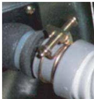
Clamp the Flexible Drain Hose Connection
