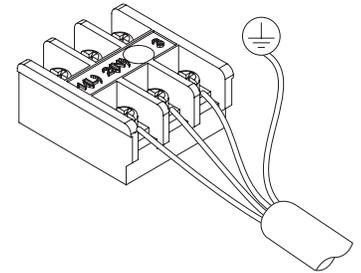
Figure 95: Proper and Improper Power Wiring Connections.
