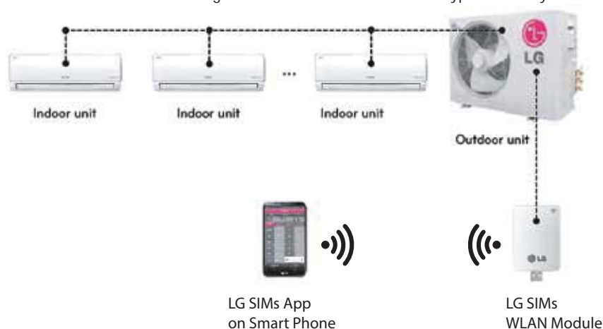
Figure 106: SIMS WLAN Module to Typical DFS System
