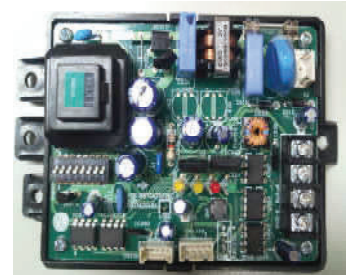
Figure 94: PI-485 Board (Appearance will differ depending on model).
