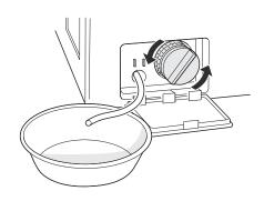
Clean the pump filter and opening.
