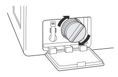
Close the drain pump filter cover.
