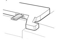
**5** Press and hold the **Freezer** button for three seconds while continuing to hold your phone to the speaker.
