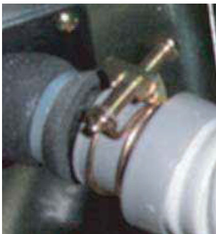
Clamp the Flexible Drain Hose Connection
