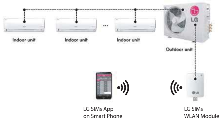
Figure 106: SIMS WLAN Module to Typical DFS System
