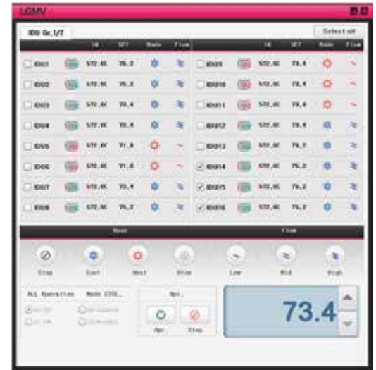
Figure 103: MV Control Indoor Units Screen
