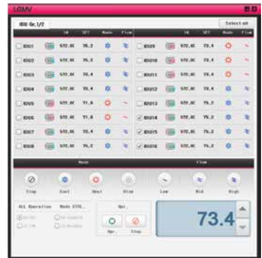
Figure 61: MV Control Indoor Units Screen.
