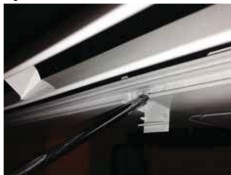
Figure 89: Remove (and Reattachment) Bottom Panel
