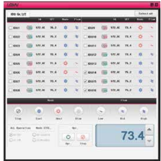
Figure 111: MV Control Indoor Units Screen
