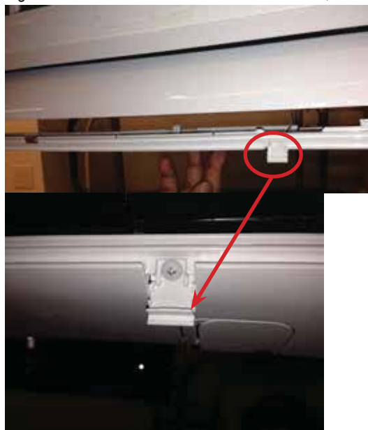
Figure 88: Remove Screws from Bottom Panel
