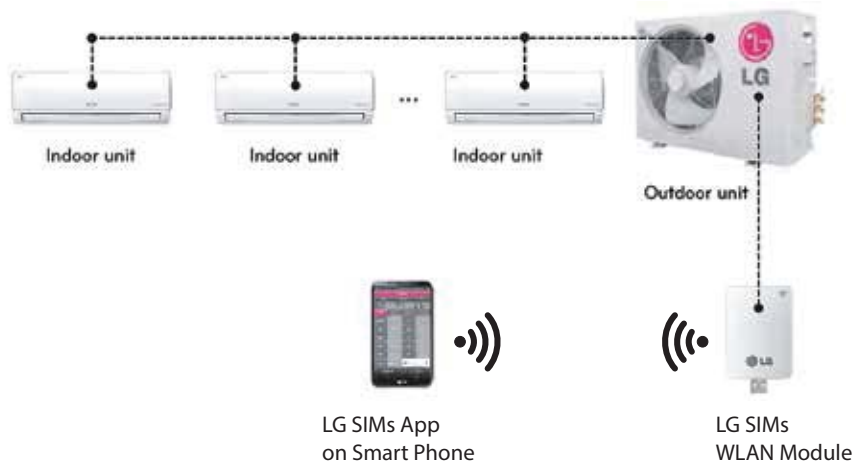
Figure 114: SIMs WLAN Module to Typical DFS System
