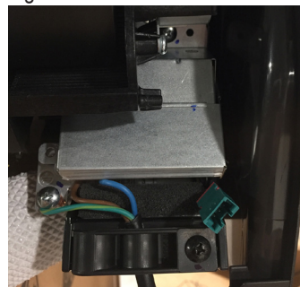
Figure 82: Terminal Cover Down.
