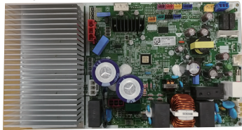
LMU183HV (18 kBtu/h) and LMU243HV (24 kBtu/h) Main PCB
