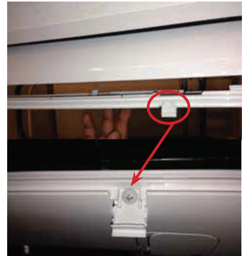
Figure 91: Reattaching the Screws on the Bottom Panel.
