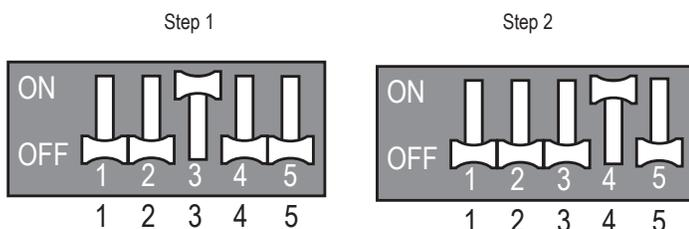
Figure 116: LMU183-243-303-363HV Wiring Error Check DIP Switch Setting.
