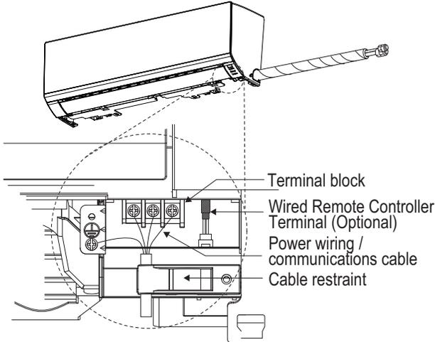
Figure 78: Connecting the Power Wiring / Communication Cable to the HVT Indoor Unit Terminal Block - Back View.
