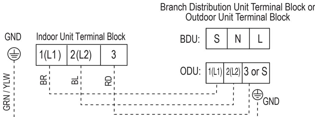
Figure 80: Indoor Unit to Outdoor Unit / Branch Distribution Unit Terminal Connections—LMN249HVT.
