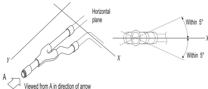
Figure 58: Y-Branch Port Identifier Diagram.
