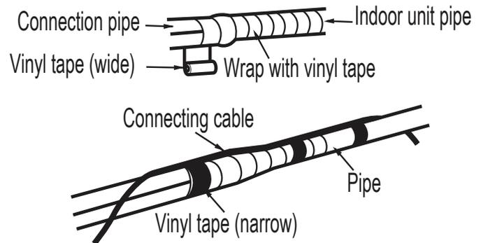
Figure 35: Cutaway of Proper Pipe and Cable Bundling.
