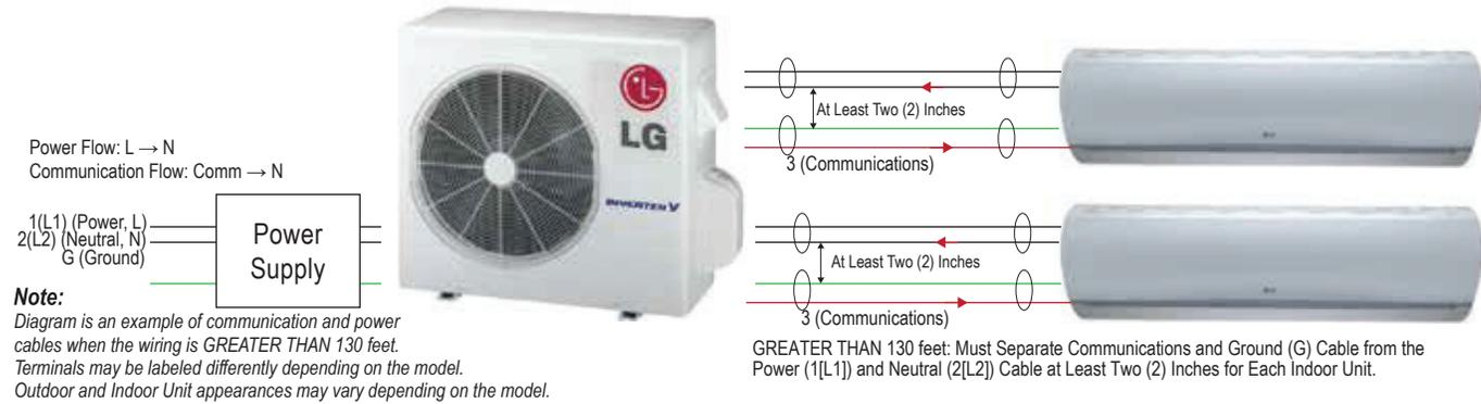
Figure 66: Schematic of a Multi F MAX with LGRED System When the Wiring is GREATER THAN 130 Feet.
