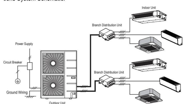
Figure 83: Multi F LMU183HV System Power Wiring and Communications Cable.
