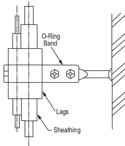
Figure 40: One-Point Down-Stop Support (>441 lbs.).
