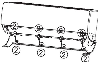
Figure 95: Snapping the Top Left and Right Sides (Step 4).
