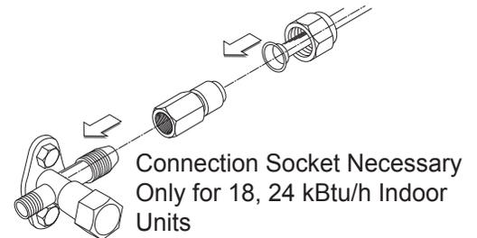
Figure 39: Connection Socket Diagram, External View.
