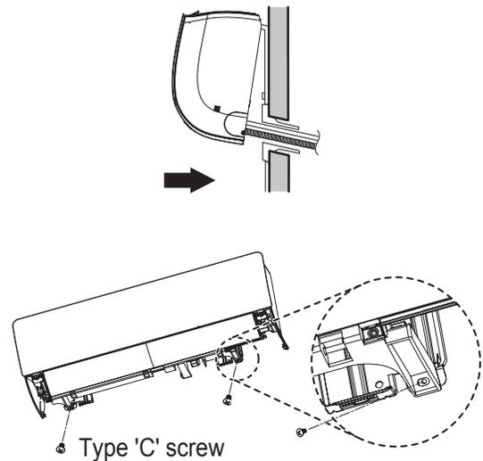
6. Finish the installation by completely securing the indoor unit to the installation plate using the factory-supplied screws (screw placement will vary depending on indoor unit model).
