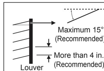
Figure 9: Using “S” Type Louvers.
