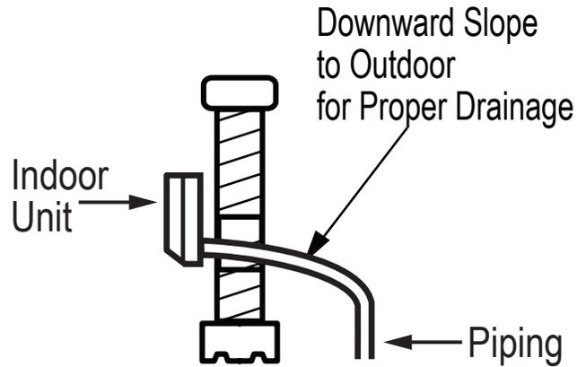
Figure 50: HVT and HSV5 Outdoor Unit Drain Hose Extension.
