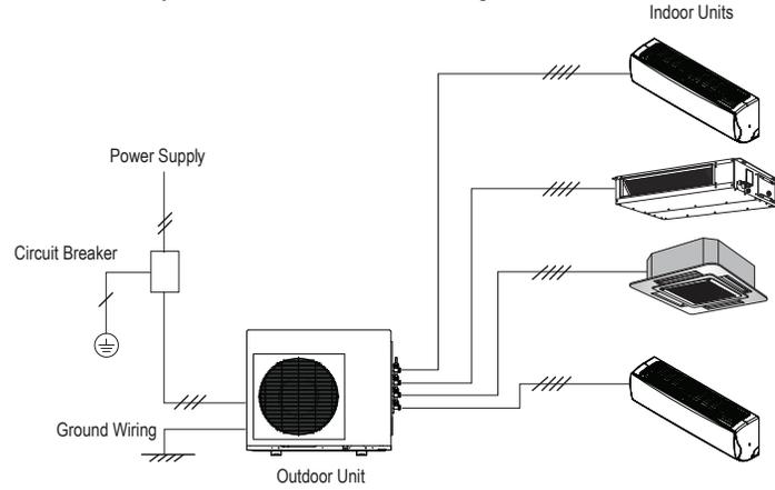
Figure 64: Typical Multi F MAX with LGRED System General Power / Communications System Schematic When Wiring is Less Than 130 Feet.
