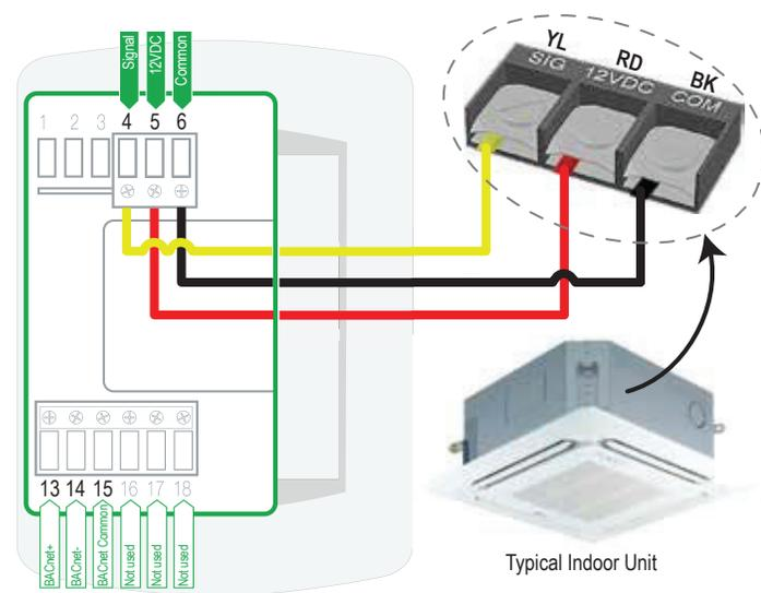
Figure 68: Another Example of Indoor Unit to Zone Controller Connection.
