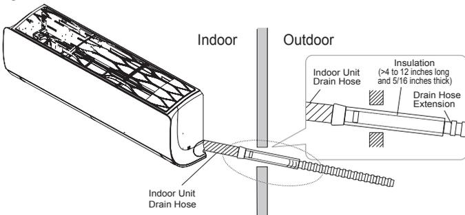
Figure 51: Inserting the Drain Hose >2 inches Into the Field-Supplied Drain Pipe.
