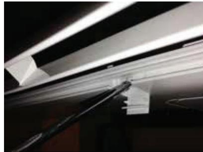
Figure 91: Reattaching the Screws on the Bottom Panel.
