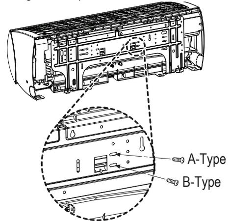
Figure 13: Installation Plate for LSN180HSV5 and LMN249HVT Indoor Units.
