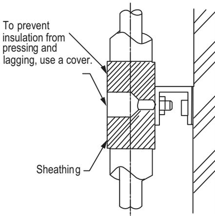
Figure 39: O-Ring Band Support with an Insulated Pipe.
