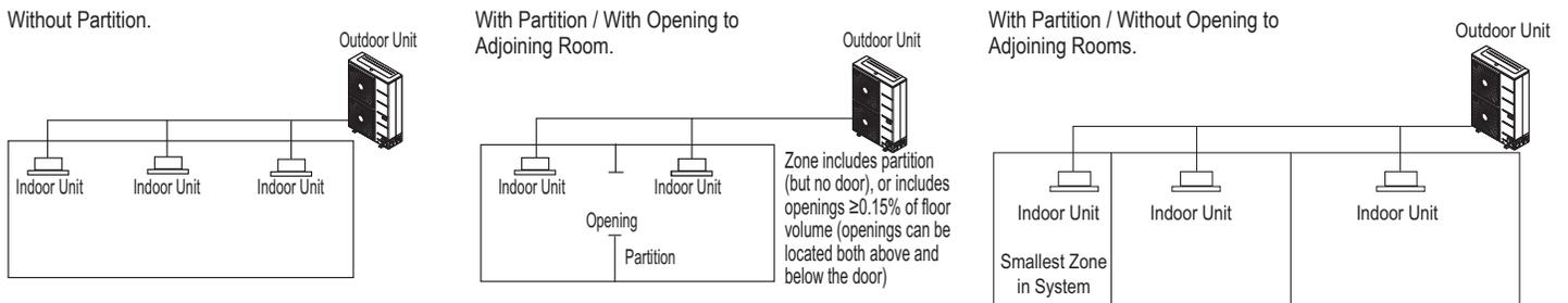
Figure 107: Example of Acceptable Ventilation Methods.
