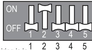
Figure 117: LMU481-541-601HV Wiring Error Check DIP Switch Setting.
