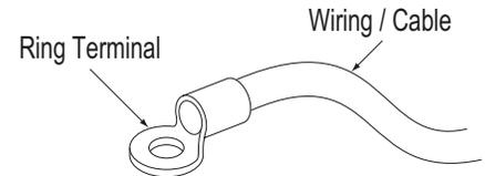
Figure 74: Adding a Ring Terminal to the Wiring.
