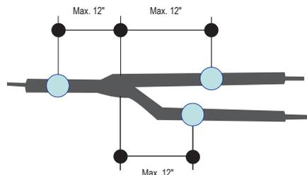
Figure 34: Pipe Support at Header Fitting.
