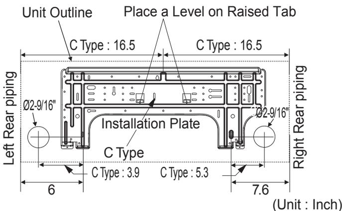
Figure 10: General Wall Mount Indoor Unit Installation Plate—Side View (Example Only. Appearances Will Vary Depending on Model).
