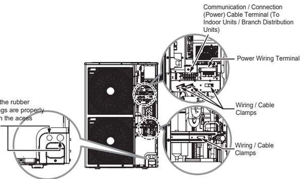
Figure 90: Connecting the Power Wiring / Communications Cables to the Outdoor Unit (LMU601HV).
