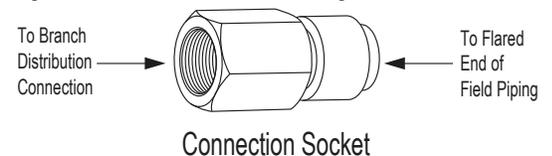
Figure 44: Close Up of Branch Distribution to Indoor Unit Piping Connections.
