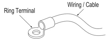
Figure 58: Adding a Ring Terminal to the Wiring.
