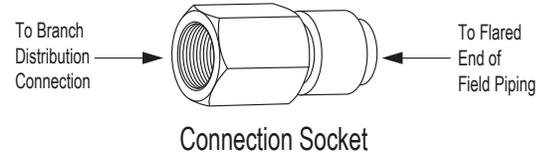
Figure 55: Close Up of Branch Distribution to Indoor Unit Piping Connections.
