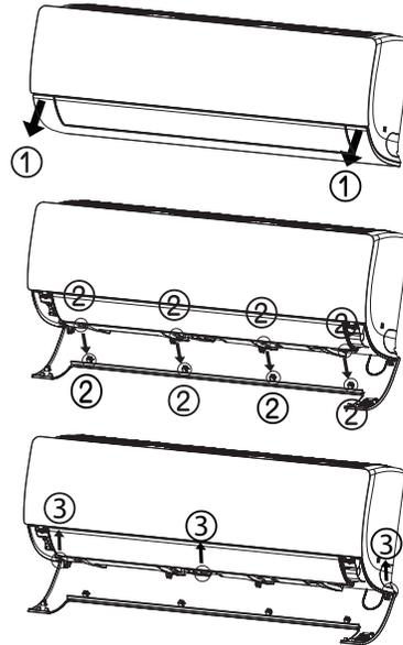
Figure 18: Removing the HSV5 Bottom Cover (Appearances Will Vary Depending on Indoor Unit Model).
