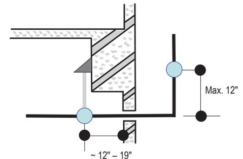
Figure 32: Pipe Support at Indoor Unit.
