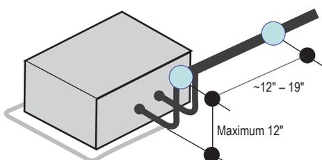
Figure 33: Pipe Support at Y-branch Fitting.
