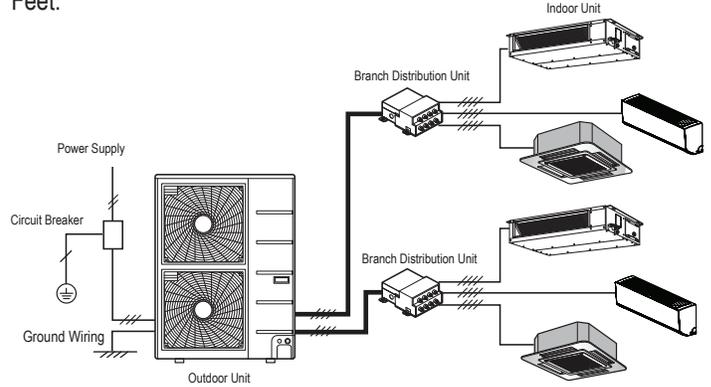
Figure 65: Schematic of a Multi F with LGRED System When the Wiring is GREATER THAN 130 Feet.
