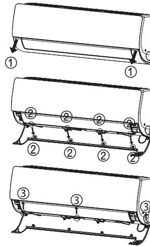
Figure 82: Removing the Bottom Cover (Appearances Will Vary Depending on Indoor Unit Model).
