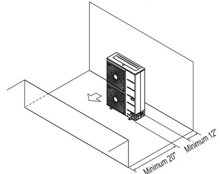
Where there are obstacles above, and on both suction and discharge sides (discharge side obstacle is higher than the outdoor unit).
