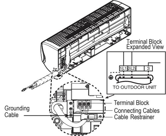
Figure 79: Indoor Unit to Outdoor Unit / Branch Distribution Unit Terminal Connections—LMN079HVT and LMN159HVT.
