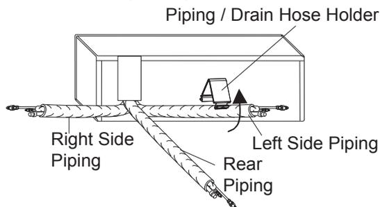
Figure 28: Bending Piping at Rear of Indoor Unit.
