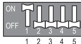
Figure 115: LMU481-541-601HV Forced Cooling DIP Switch Setting.
