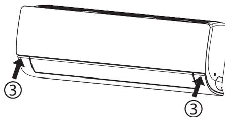
Figure 96: Checking that All Attachment Locations Are Secure (Step 5).
