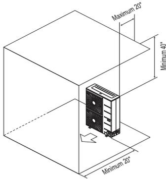
Where there are obstacles on both suction and discharge sides (discharge side obstacle is higher than the outdoor unit).
