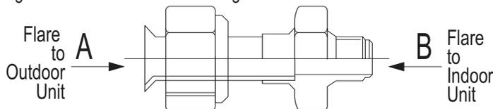
Figure 49: Performing Connections.
