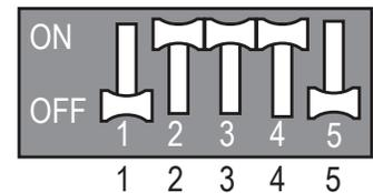
Figure 123: LMU481-541-601HV Saving Power Consumption with Mode Lock DIP Switch Settings.
