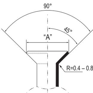
Flared Connection Dimensions / Tightening Torque.
