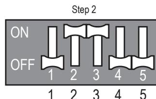
Figure 125: LMU481-541-601HV Night Quiet Mode DIP Switch Settings.
