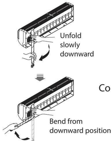
4. From the rear of the indoor unit, carefully bend the copper pipe tubing holder away from the unit to expose for conduit bracket installation area.
