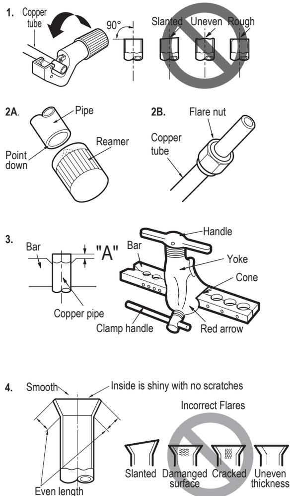
Figure 16: Dimensions of the Flare
