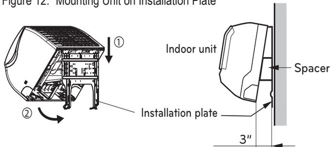
Figure 13: Mounting Unit on Installation Plate
