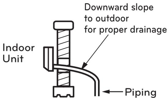
Figure 36: Correct Slope Angle for Drain Hose
