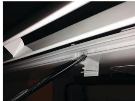
Figure 62: Remove (and Reattachment) Bottom Panel
