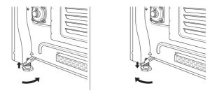
Use a level to check your adjustments. Place the level diagonally on the oven rack, and check each direction for level.
