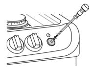
Hold the valve shaft with one hand while turning the screw to adjust with the other.
