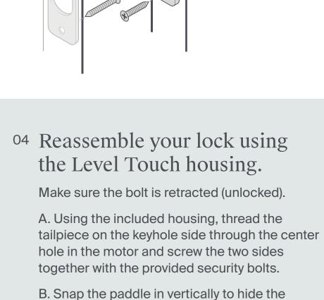
\*To disassemble in the future, use a paperclip or pen to press the small hole on the bottom of the paddle,
