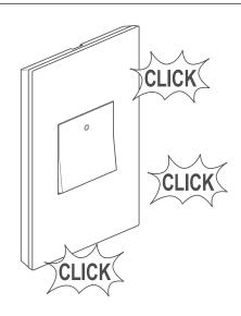
NOTE – To remove wall plate, insert a small, flat screwdriver in notches on wall plate and twist gently to pry from frame.
