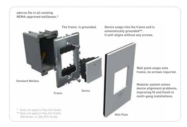
Devices simply snap into the frame from the front. During installation, screw the frame to the box, then pull the wires through the frame and wire the device. Then, simply snap the device into the frame.
