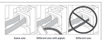
Carefully fold wires into box. Snap outlet into frame.
