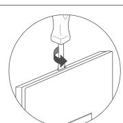
NOTE - To remove wall plate, insert a small, flat screwdriver in notches on wall plate and twist gently to pry from frame.
