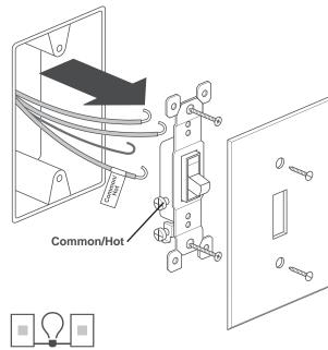
3-Way In a 3-Way circuit, identify the Common/Hot wire connected to the terminal
