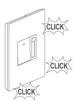
**NOTE** – To remove wall plate, insert a small, flat screwdriver in notches on wall plate and twist gently to pry from frame.
