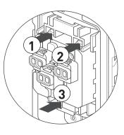
Snap wall plate to frame. There are three click-stops to adjust the fit of the wall plate to the outlet and the wall.
