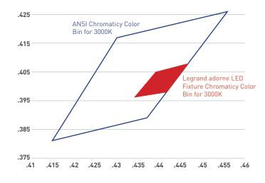
adorne individual LEDs are specifically selected to ensure fixture output CCT uniformity within a range of less than 100. This tight manufacturing assurance process ensures that variations inherent in the LED chip manufacturing process do not compromise reliable light quality.
