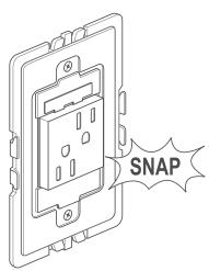
NOTE - If you need to remove outlet after snapping into frame, first remove frame from wall box to access the three locking tabs on the back of the outlet. Insert a flat screwdriver to depress tabs as you apply pressure to push outlet out.
