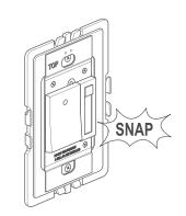
NOTE – If you need to remove dimmer after snapping into frame, first remove frame from wall box to access the four locking tabs on the back of the dimmer. Insert a flat screwdriver to depress tabs as you apply pressure to push dimmer out.
