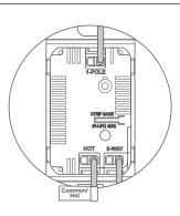
NOTE - In a 3-Way installation, use one dimmer and one switch. Do NOT use two dimmers.
