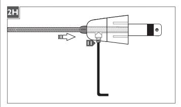
II Firmly tighten the set screw on the conical connector.
