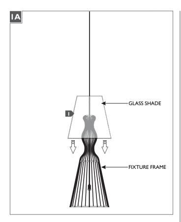
II Slip the cord through the glass shade and gently lower the glass shade onto the fixture frame.
