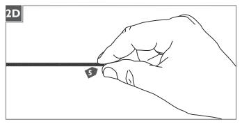
Gently twist the end of the coaxial cable between thumb and forefinger.
