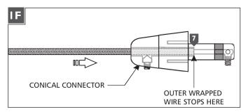
Feed and push the coaxial cable into the conical connector. The coaxial cable will come to a stop point after being inserted 3/4" into the conical connector.
