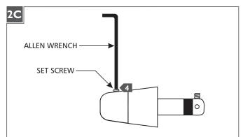
Back out (do not remove) the set screw on the conical connector with the provided Allen wrench.
