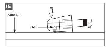
Tap the conical connector on a hard surface with the set screw facing down, so the plate inside drops into place.
