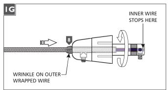
Reep pushing the coaxial cable into the connector while rotating the connector to ease feeding the inner wire into the tip of the connector. The outer wrapped wire will start wrinkling while being inserted another 1/2" into the connector.
