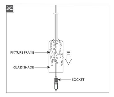
Gently lower the fixture frame and glass shade until they rest properly on the socket assembly.
